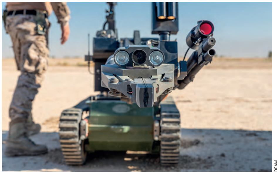
Explosive ordnance disposal robot used by the Armed Forces to locate, identify and handle suspicious devices.
