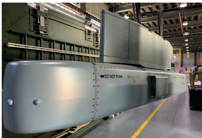
Pod for electronic reconnaissance missions for Air Force F-18 fighters.
