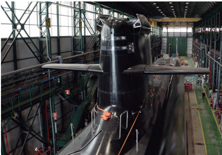
The next step will be the installation of masts (communications, electronic warfare, radar and snorkel) and periscopes on the submarine's sail.
